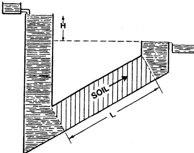
Figure 7. Water movement as a result of potential difference.
