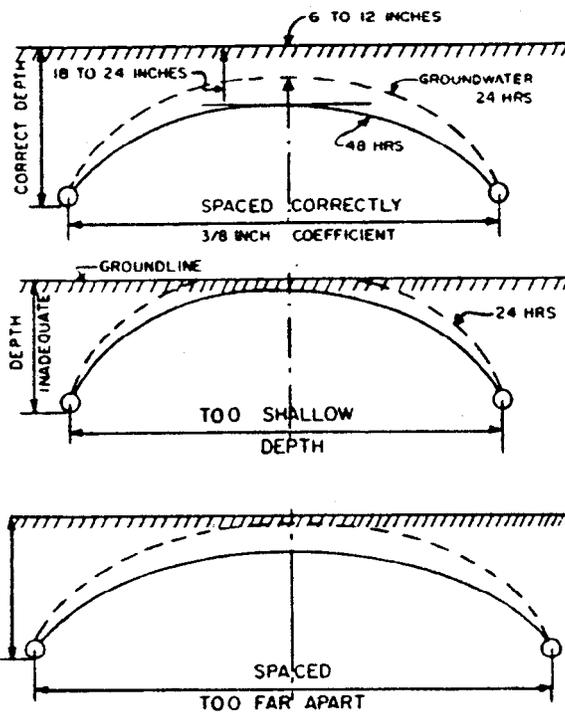
Figure 11. Depth and spacing relationships.
