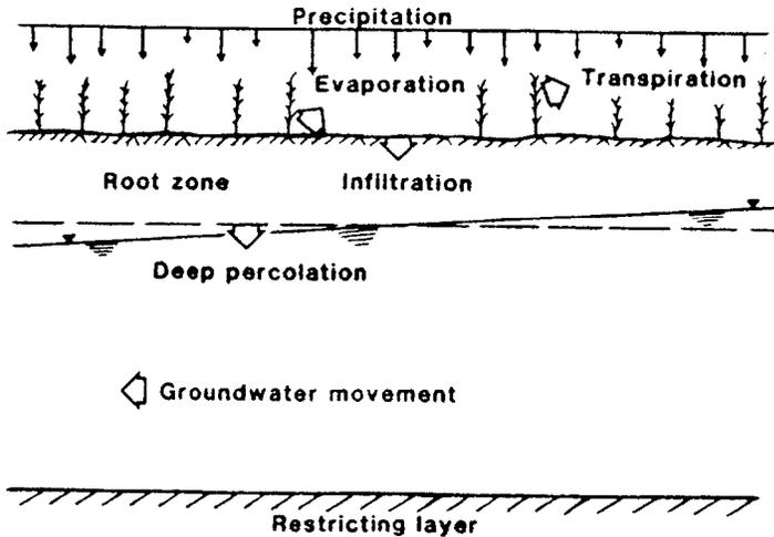
Figure 5. Water movement in soils.
