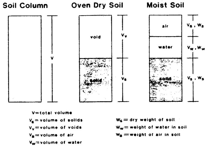
Figure 1. Volumetric relationships of soil.
